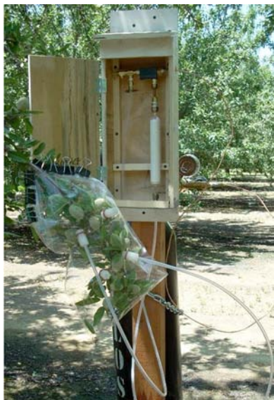
Figure 1. Closed volatile collection system used to collect in situ hull split volatiles from an enclosed almond branch.
